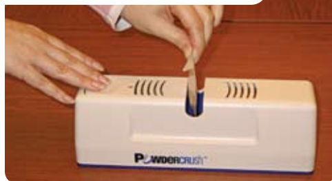
6. Strike the pouch by pressing the button.
