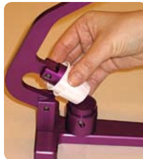
10. Place the stacked containers on the anvil.
